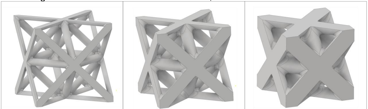
Figure A3 - Octet-truss structure with 10%, 25% and 50% of volume fill
