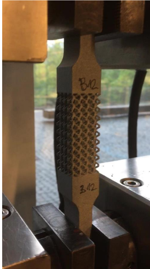
Figure 21 - Tensile test specimen with BCC structure positioned in testing machine.
