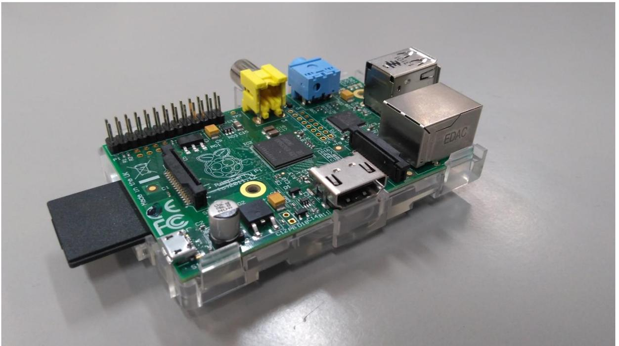
Figura 1: Raspberry Pi Modelo B
