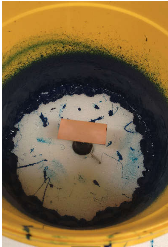
Figure 18 – PCB board and a 12V DC Motor before applying the liquid photoresist
