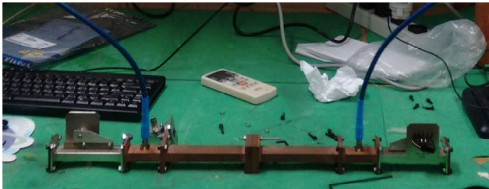
Figure 23 – Set up to measure the S-Parameters with the cells inside the waveguide
